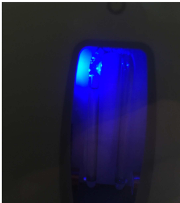
Figure 07: Main fermentation sample unfiltered and non-degassed in the measurement chamber. The released CO 2 is clear to see in the upper part of the oscillating U-tube. Sample label #3
